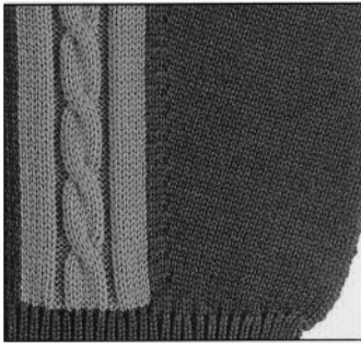
Widening with split-stitch (latch-type needle)
