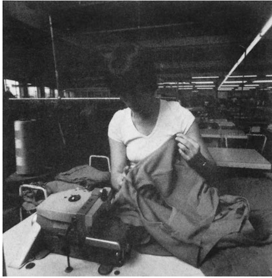
Fig. 6.3 Overlock seaming [Corah].
