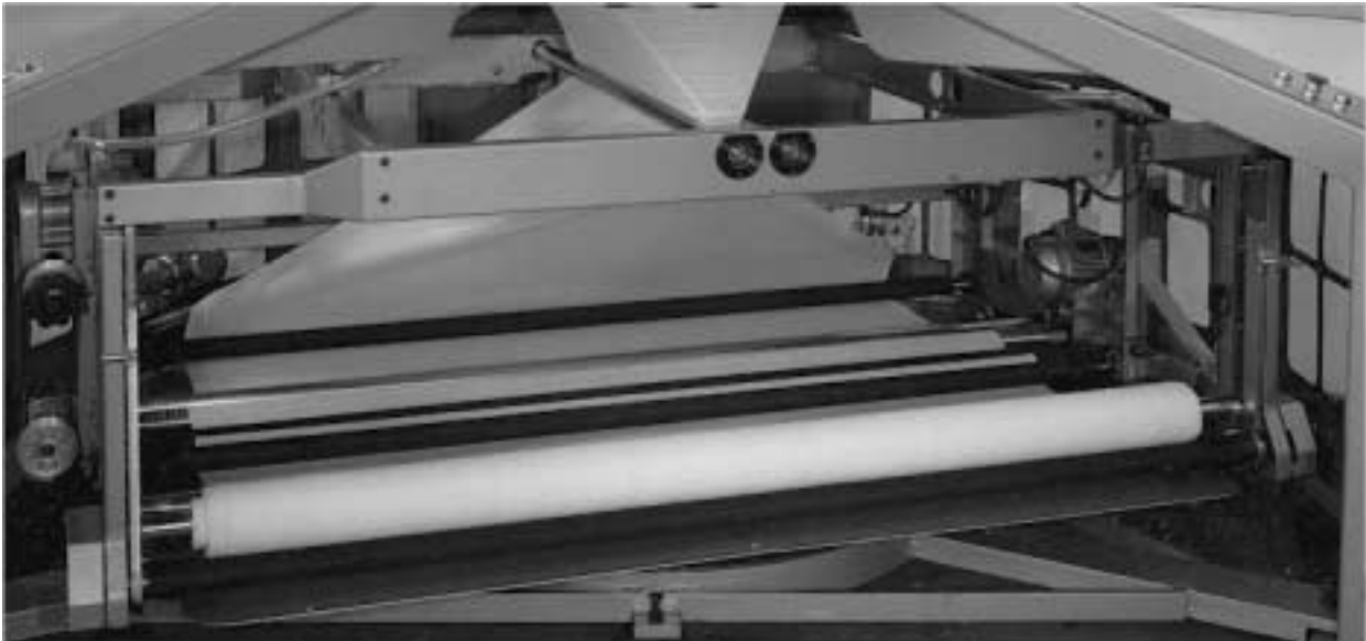
Picture 100 – Open-width winding motion
