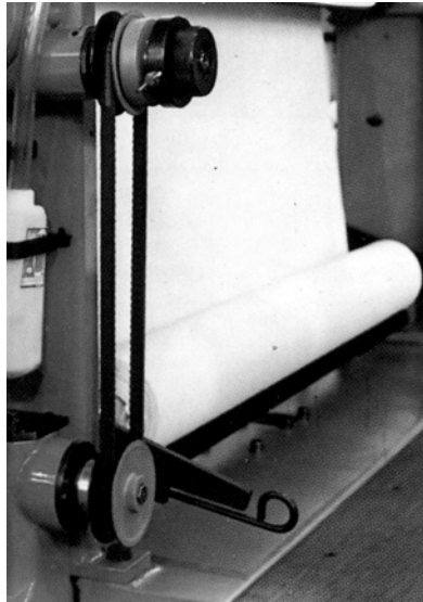
Picture 99 – Clutch connection between the winding roller and the take-down motion rollers
