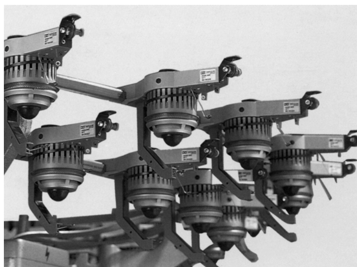
Picture 79 – Yarn feeding accumulator
