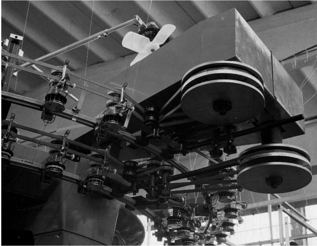
Picture 80 – Positive belt feeding system
